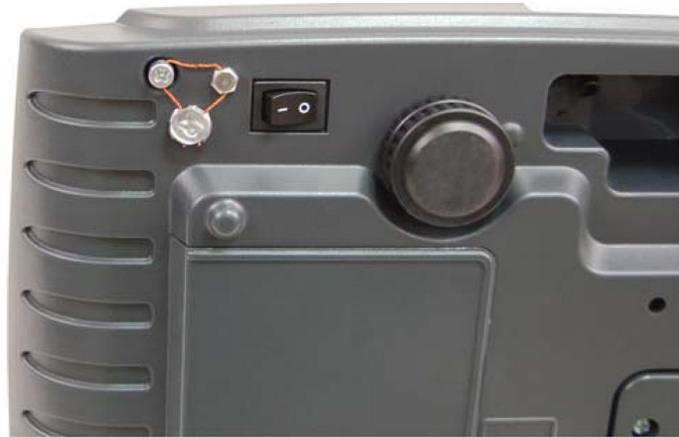
A wire seal is passed through the holes in two sealing screws mounted on the bottom of the scale.
